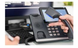
**VAC IP PBX** is a private telephone switching system within an enterprise to converge data and voice networks. This means that Internet access, VoIP communications and traditional telephone communications are all possible using a single line. This provides flexibility as an enterprise grows & can also reduce long term operation and maintenance costs.
